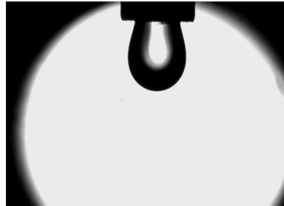
Drop of water-rich phase in the CO 2 -rich phase at 68F and 862psig
